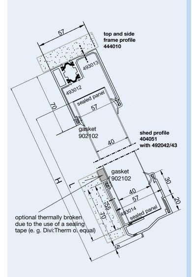
Calculation of panel length:  $\mathbf{L}$  in mm = Height  $\mathbf{H}$  in mm - 55 mm
