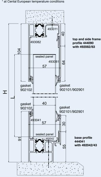
Calculation of panel length:  ${f L}$  in in mm = Height  ${f H}$  in mm - 110 mm
