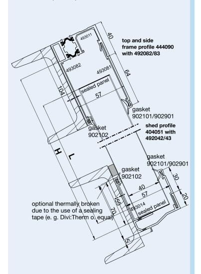
Calculation of panel length:  $\mathbf{L}$  in mm = Height  $\mathbf{H}$  in mm - 75 mm
