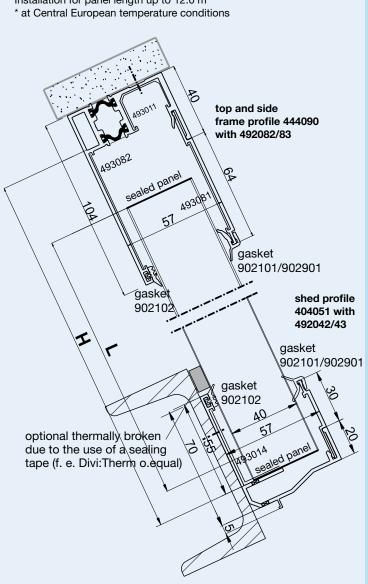
Calculation of panel length: L in mm = Height H in mm - 75 mm
