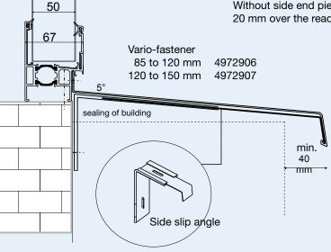
With a projection/profile depth of more than 150 mm additional fasteners (Vario-fastener or Clinker-fastener) on the structure are necessary. (every 800 to 1,000 mm)
