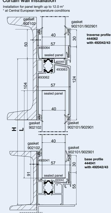
We recommend to support the base profile for panel length starting from  $7.00\ m$
