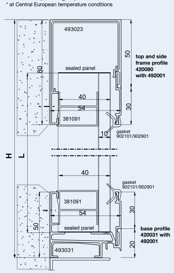
We recommend to support the base profile for panel length starting from 7.50 m.
