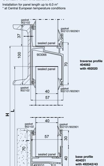
Calculation of panel length:  $\bf L$  in mm = Height  $\bf H$  in mm less 60 mm at H > = 1,500 mm less 70 mm at H < = 1,500 mm
