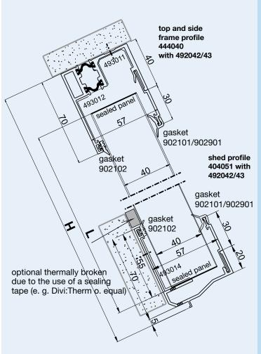
Calculation of panel length: L in mm = Height H in mm - 55 mm
