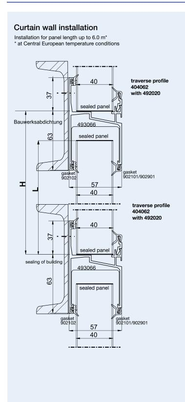
Calculation of panel length: L in mm = Height H in mm - 30 mm
