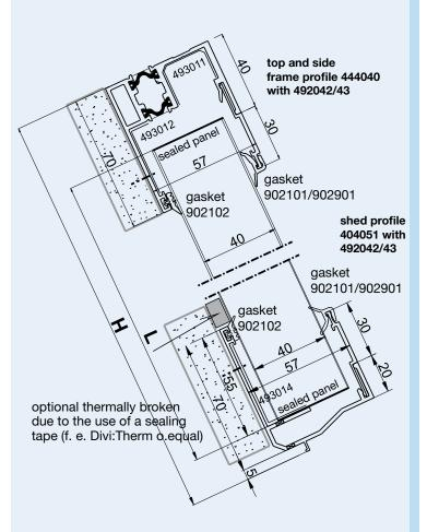
Calculation of panel length:  $\mathbf{L}$  in mm = Height  $\mathbf{H}$  in mm - 55 mm
