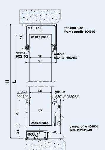
Calculation of panel length:  $\bf L$  in mm = Height  $\bf H$  in mm less 50 mm at H > = 1,500 mm less 55 mm at H < = 1,500 mm
