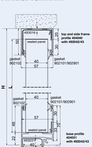
Calculation of panel length: **L** in mm = Height **H** in mm less 50 mm at H > = 1,500 mm
