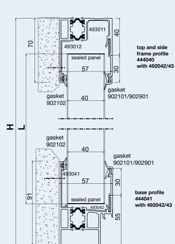
Calculation of panel length:  ${f L}$  in mm = Height  ${f H}$  in mm - 90 mm
