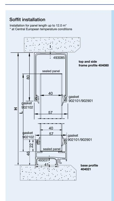
Calculation of panel length: L in mm = Height H in mm less 55 mm at H > = 1,500 mm
