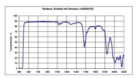
The measurement of the transmission values was carried out with application of a natural day light lamp of 20.000 Lux in connection with a lux meter Lightmeter MS 1000-300 - measuring range 200 to 50.000 LUX) exemplarily on a 1 mm thick PC.
