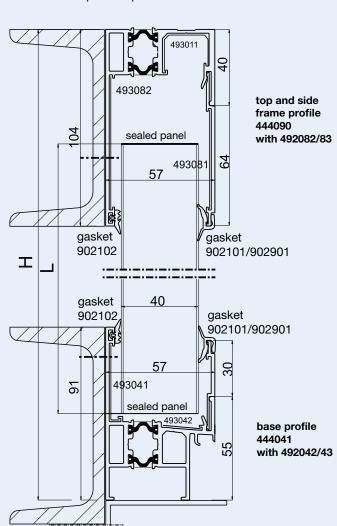
We recommend to support the base profile for panel length starting from 7.00 m
